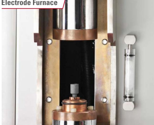
A graphite crucible will be pressed between two electrodes and heated up, in the furnace by using max. 1000 A power. The temperature of the furnace is PC controlled and might reach up to a maximum of 3000 °C.
