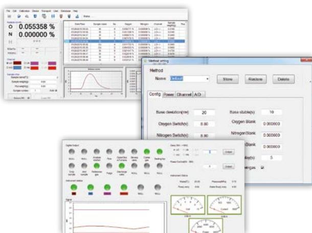
The NCS operation software is designed for the easy operation of our elemental analysers. It incorporates a desktop for the sample analysis with data transmission as well as the set-up of different methods and user profiles.
