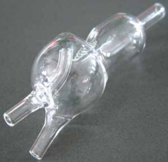
▲ Gas and Liquid Separator
