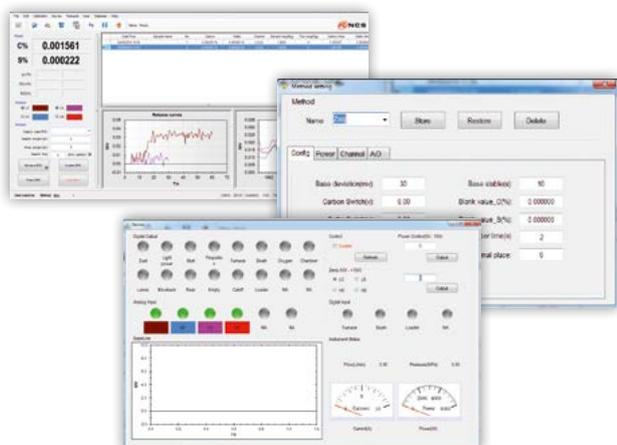
The NCS operation software is designed for the easy operation of our elemental analysers. It incorporates a desktop for the sample analysis with data transmission as well as the set-up of different methods and user profiles.
