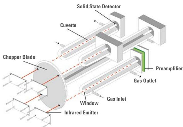
The IR system is designed for a precise operation with low maintenance. The constantly active IR emitter is providing a low-noise signal.
