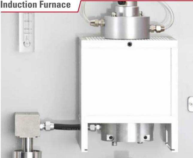
The furnace will heat up the sample by inductivity up to 2200 °C. The power of this process is controlled by the PC and might reach up to 2.2 kVA.
